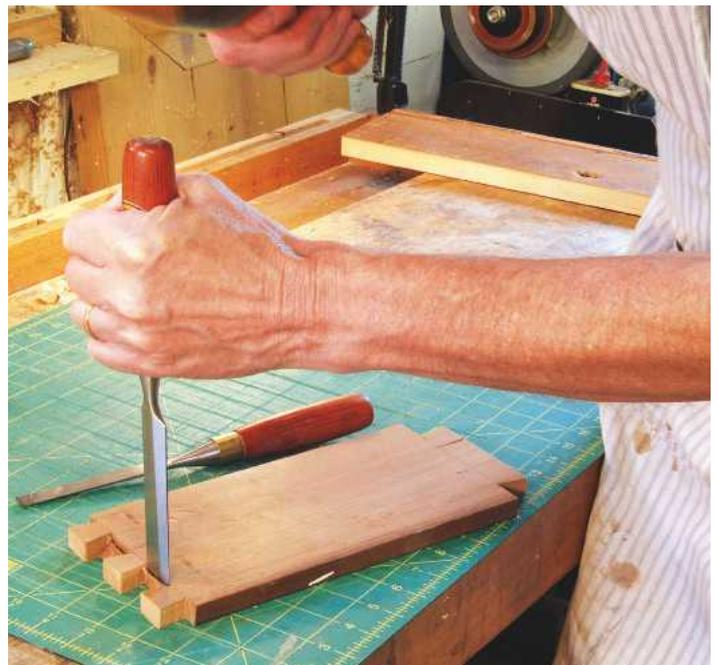
▲ Pic.9 Cleaning back to the shoulder line of the tails with a vertical cut
